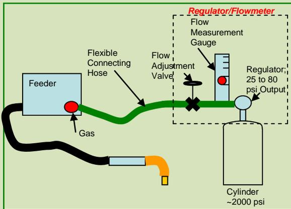
A small restriction orifice or a valve is used to control the gas flow. Typical regulator outlet pressures are from 25 to 80 psi. For CO<sub>2</sub> shielding 80 psi is often used to help prevent ice formation. These higher pressures needed to provide automatic flow compensation for restrictions occurring during use. Anything lower will eliminate this important function (See Reference 3.)
